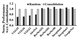
**Figure 3:** 4 concurrent 8-worker jobs with different placement schemes. The performance values are normalized by the value of the consolidation scheme. We use the median value from 10 (20) runs for consolidation (random) scheme.
