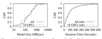
Figure 16: The CDF of DL modelFigure 17: The CDF of averagesizes being trained.iteration time per job.
