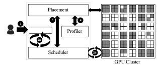
Figure 6: Tiresias components and their interactions. Job lifecycle under Tiresias is described in Section 3.1. In this figure, each machine has four GPUs; shaded ones represent GPUs in use.
