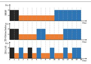
Figure 7: Time sequence of three jobs with three different twodimensional scheduling algorithms. Job 1 (black) is (2, 2), job 2 (orange) is (1,8), and job 3 (blue) is (2,6). The first value in each tuple is the number of GPUs while the second is duration. The scheduling interval is one unit of time. The 2D-Gittins index values for this example are shown in Appendix C. Job index is used to break ties.
