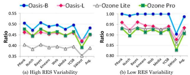
Fig. 14. The ratio of green energy usage to overall power consumption. Ozone Pro has relatively higher dependence on grid power.
