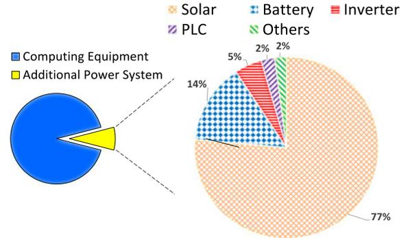
Fig. 17. Cost breakdown of the Oasis node scaled to a 40U standard rack of moderate power density (<10 KW).
