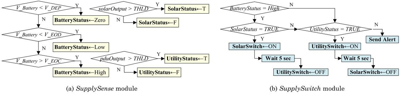
Fig. 4. The control flow of power supply switching. Oasis in autonomous mode uses two atomic modules to control the system. (DEP - Depletion; EOD - End of Discharge; EOC - End of Charge;  $V_{EOC} > V_{EOD} > V_{DEP}$ ).
