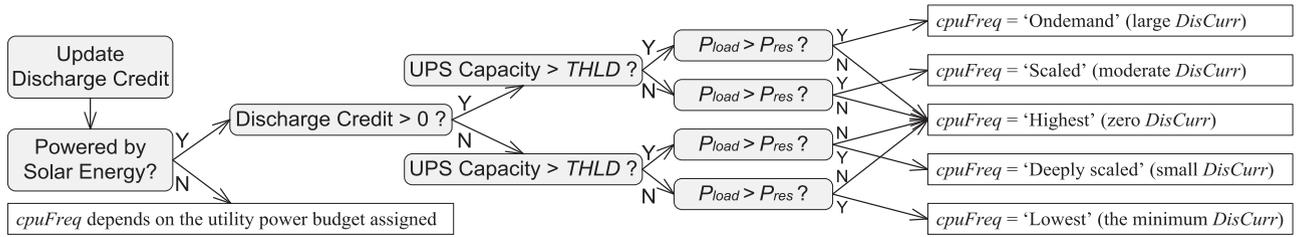
Fig. 5. The decision tree of Ozone performance management. THLD: Preset threshold of the state of charge; cpuFreq: Server frequency mode; DisCurr: Battery discharge current.
