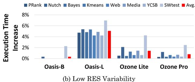
Fig. 11. The execution time increase due to server performance scaling.
