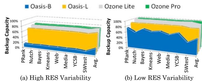
Fig. 13. The average battery backup capacity. Ozone maintains high backup time due to its better battery capacity management capability.
