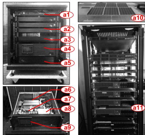
a1) network switch, a2) computing nodes, a3) front-end server, a4) power control hub, a5) In-rack battery chassis, a6) converter and inverter, a7) power supply switch, a8) PLC module, a9) HMI, a10) roof-mounted solar panels, a11) local cloud servers
