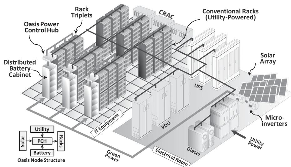
Fig. 3. Schematics of Oasis architecture. Oasis leverages the modularity of both battery systems and renewable power systems to improve scalability and economy. A power control hub is designed to coordinate utility power, solar power, and local battery.
