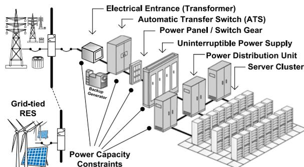
Fig. 2. Conventional datacenter power distribution system is not scale-out friendly. Facility-level green energy integration can also be cost-prohibitive and low-efficiency.
